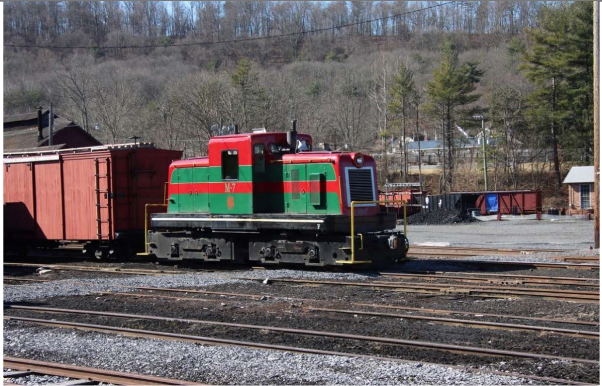
EBT'S THREE-FOOT GAUGE GENERAL ELECTRIC 50-TON DIESEL-ELECTRIC LOCOMOTIVE M-7 – Waiting for another switching assignment in the Orbisonia yard. M-7 was previously used for switching at the Algoma Steel plant in Sault Saint Marie, Ontario. The EBT purchased M-7 in 1993.
