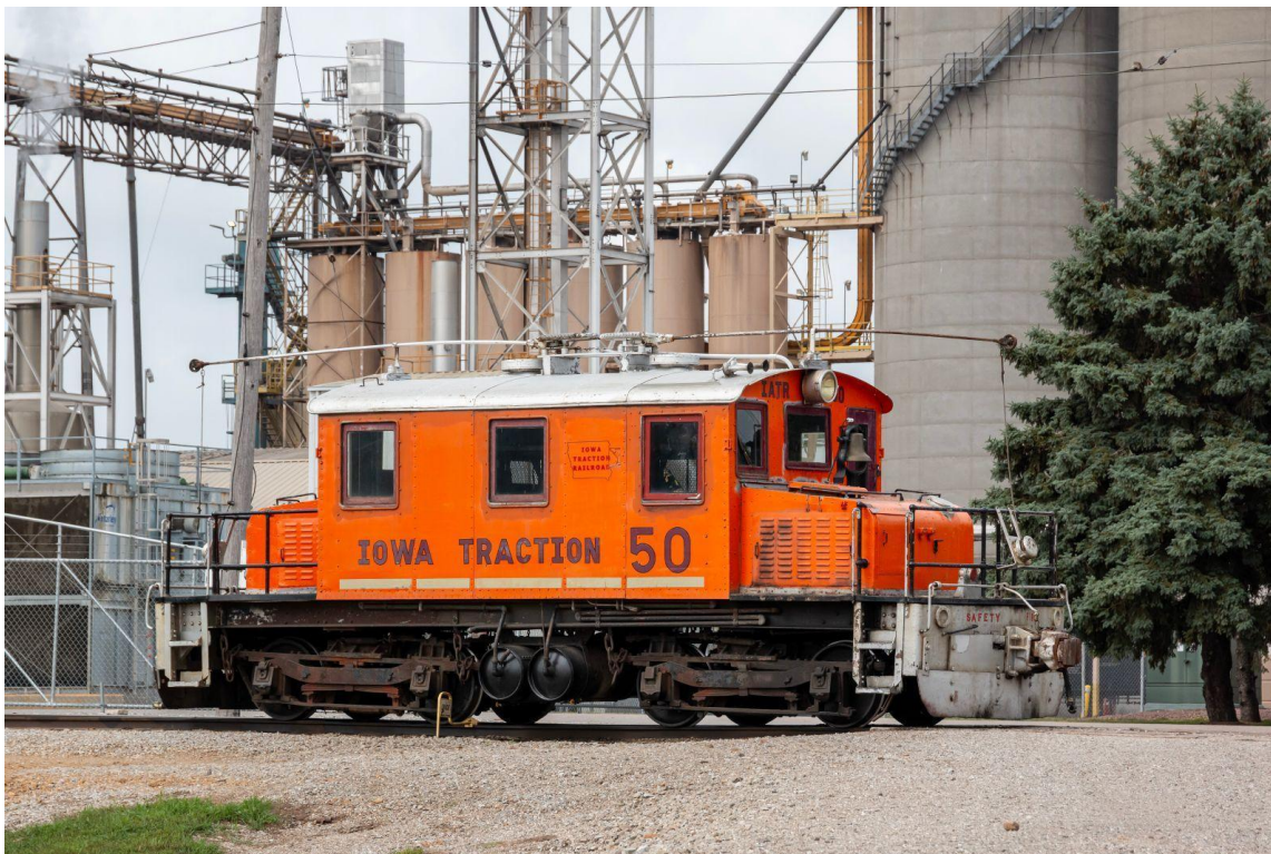
PHOTO COURTESY OF MIKE YUHAS BALDWIN STEEPLCAB ON CALL – Iowa Traction 50, a Baldwin steeplecab built in 1920, rests between assignments at an agribusiness in Mason City, Iowa.
