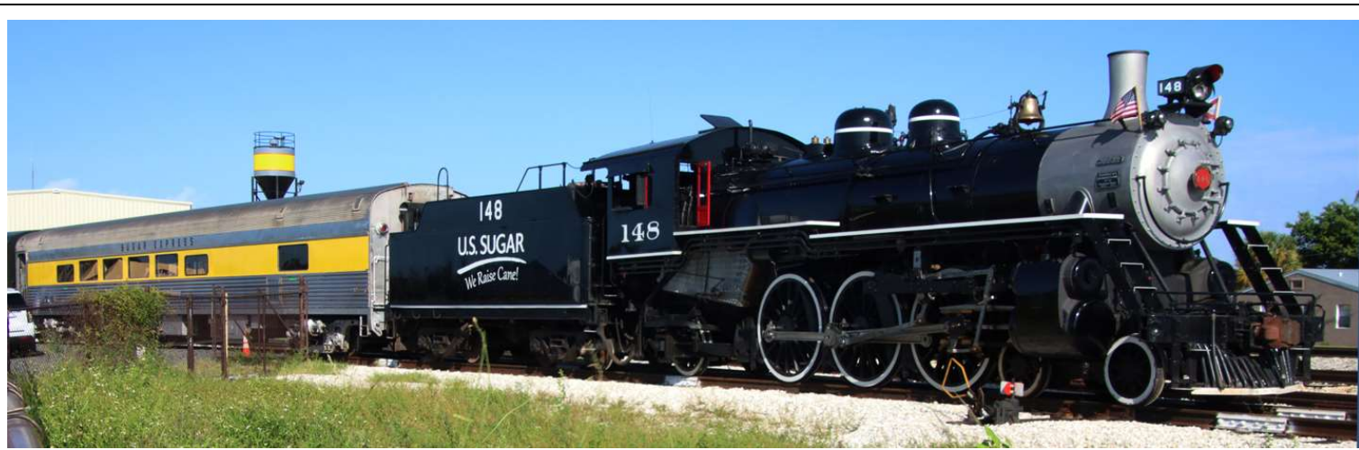
FORMER FLORIDA EAST COAST 4-6-2 NO. 148 - The power for the south-bound leg of the trip was No. 148, seen here at Clewiston just prior to boarding.
