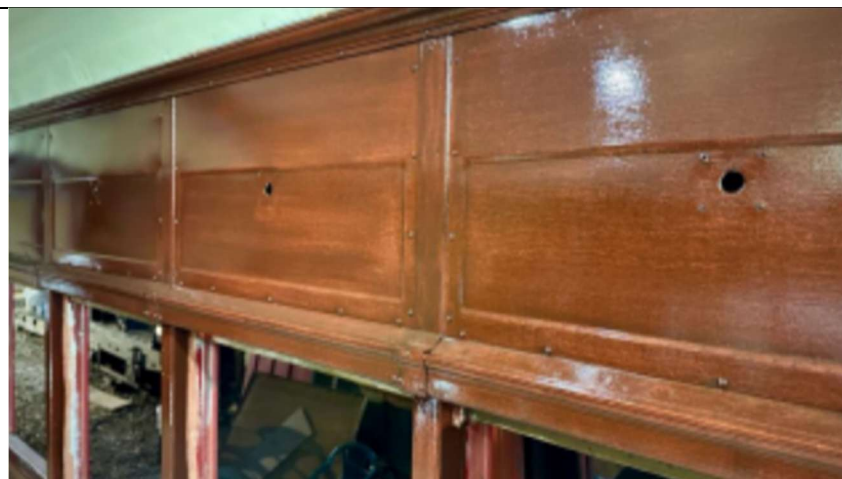
Attention to detail in the simulated highs and lows of wood is shown.
