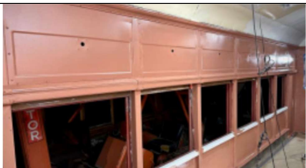
Reddened earth paint is applied to allow the highs and lows of the faux wood grain to match the car's original samples when the stain is applied.
