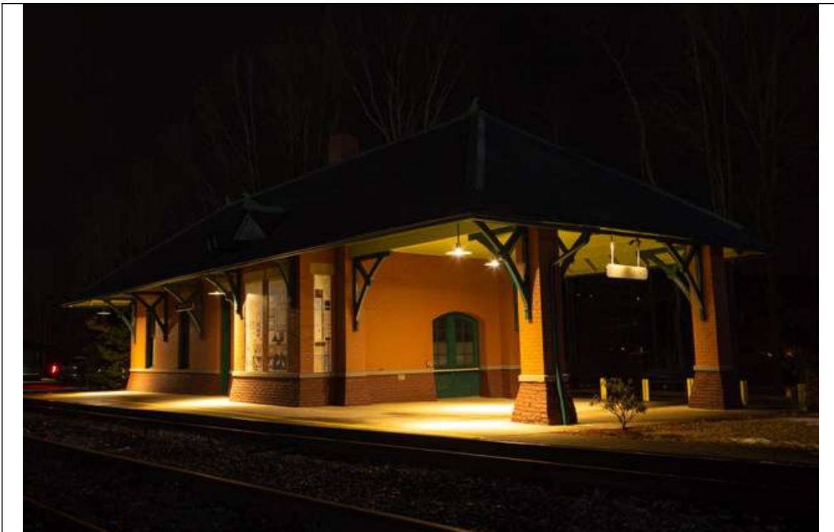
MOSCOW PASSENGER STATION - New lights have a powder coated paint finish that replicates a weathered copper patina.
