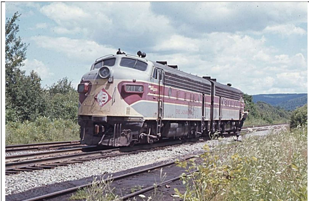
EMD F7a # DIESEL-ELECTRIC LOCOMOTIVE, JULY 21, 1974 - Erie Lackawanna Railway, Susquehanna, Pennsylvania. Sandy Burton photograph, Jersey Central Chapter NRHS Collection.
