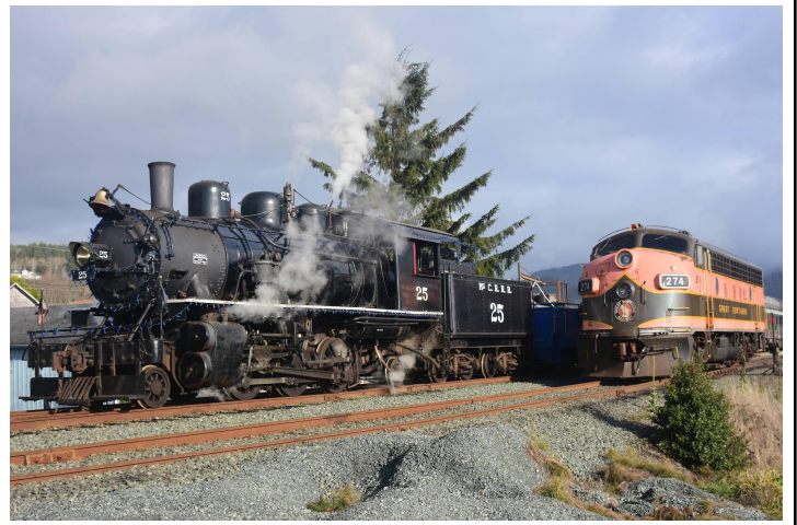
McCloud River No. 25 at Oregon Coast Scenic Railroad in Garibaldi. Built 1925 by ALCO. A 2-6-2 Prairie type. Photo on Nov. 26, 2022
