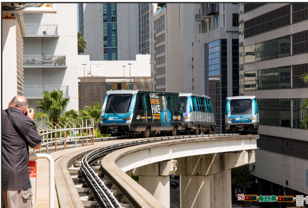
Convention delegates experienced the downtown Miami Metro Mover, a rubber-tired automated people mover. While on a stopover at the Metro Mover Knight Center station, Doug Scott photographs passing two such conveyances. Photo by Mike Yuhás.
