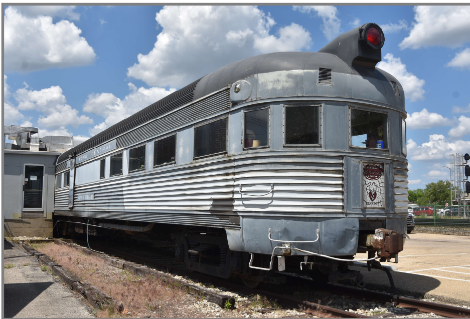
New York Central observation car "City of Elkhart", nee Chicago, Rock Island & Pacific 454 "Minnesota", built by Budd Company in 1937. It is painted for NYC, to represent similar Budd-built observation cars that were an integral part of the post-war Great Steel Fleet of streamliners. Photograph courtesy Christopher Guenzler.
