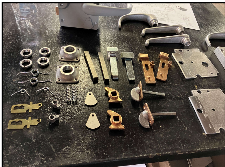
Left: The many components needed to manufacture a modern railway door handle. Right: A variety of door handles manufactured by Adlake. Photographs courtesy Elizabeth Guenzler.
