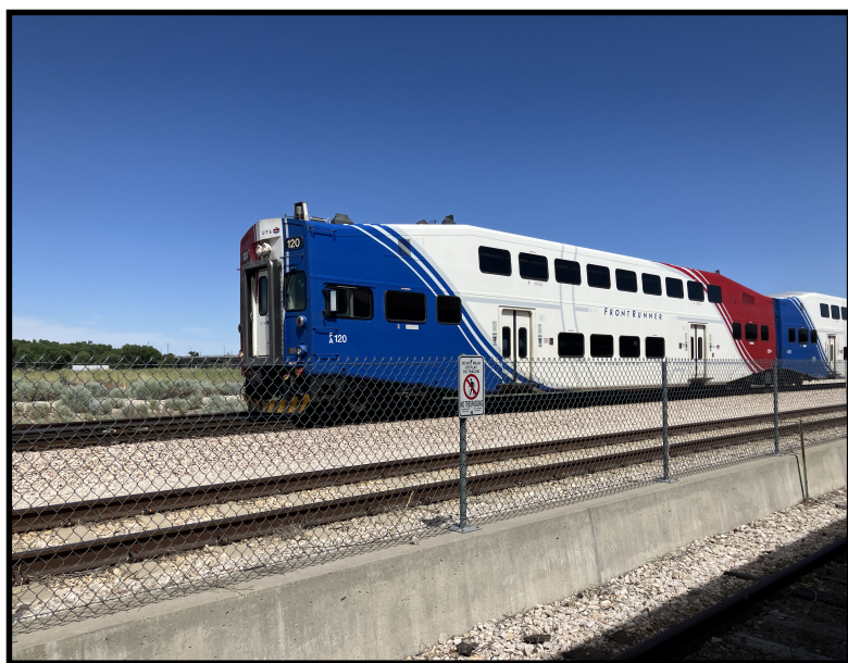
Utah Transit Authority's FrontRunner has just departed Ogden Central Station and is passing the Utah State Railroad Museum before going over the flyover as it starts the 83 mile journey to Provo. FrontRunner operates in push-pull mode; this is cab car 120 built by Bombardier and MP36PH-3C 2 built by Motive Power Industries
