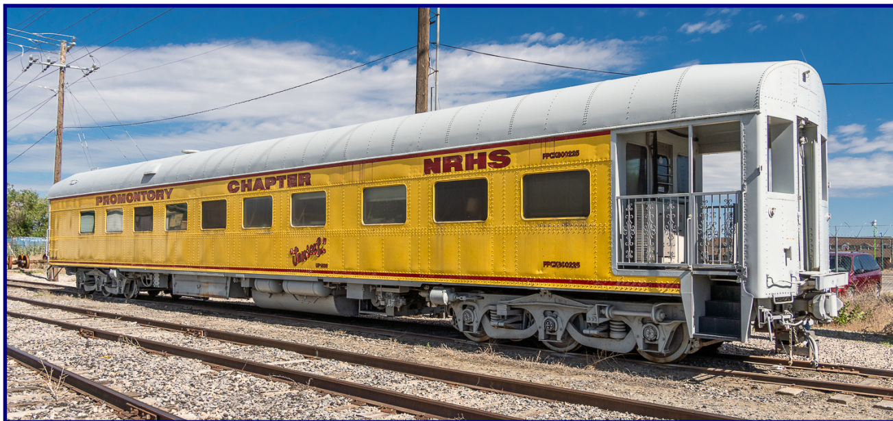
Promontory Chapter business car "Janice L", ex, Union Pacific club-dormitory 1535 1954, exx. Union Pacific club-lounge 1535 "Colorado Club" 1930 for Columbine service, nee Union Pacific club-dormitory 1535, built by Pullman Company in 1923. It was retired in 1968 and sold to a private party in Denver, then named "Janice L" in 1970. The partially-open observation platform modification was added in 1982. PPCX 800225. Photograph courtesy Doug Scott.
